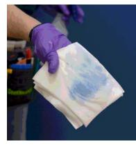
FIGURE 2 Paint Particles After First Cleaning
