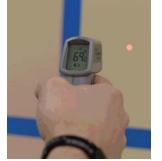
FIGURE 3 Testing Wall Temperature
